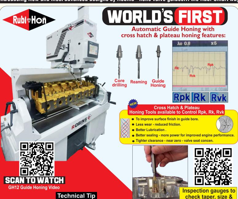
Valve Seat surface finish & concen depend on; "How precise Valve Guide Bore is?"
